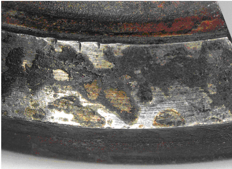
Fig.3. L12 valve after 3000 hours of operation. Magnification 10x
